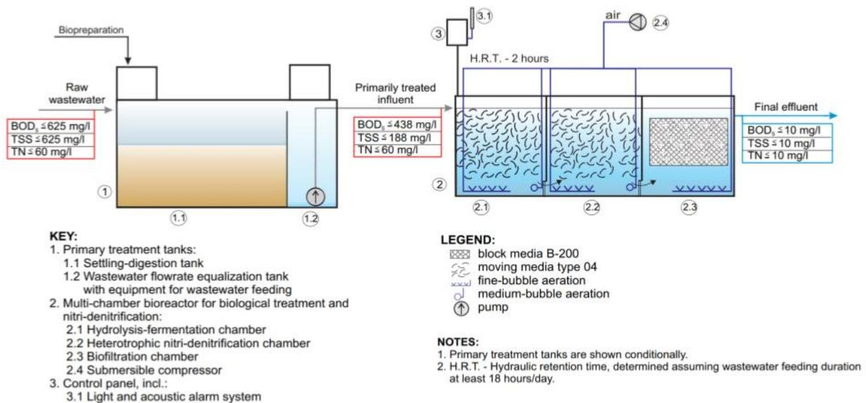
*Diagram for a commercial or mixed-use system treating very contaminated influent to a high standard.*
